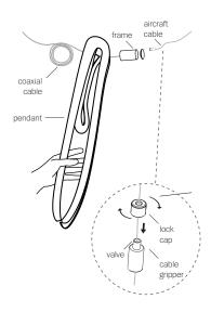
Loosen the lock cap and push the valve on the cable gripper and adjust the position of the cable gripper so that the aircraft cable is roughly the same length as the coaxial cable.
