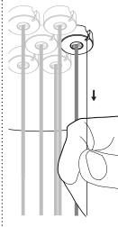
Very carefully uncoil the braided coaxial cable in a spool like manner. Insert your index fingers into opposite sides of the roll then rotate your fingers around each other to unroll the coaxial cable.
